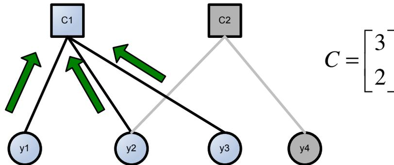
**Figure 3** Example of the averaging operation at each VFC. The vector C represents the degree of each VFC
