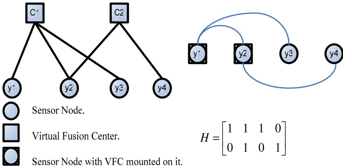
**Figure 2** Representation of WSN using Tanner graph. In this graph, C's represent VFC nodes and Y's represent sensor nodes. The matrix  $H$  denotes the routing graph.
