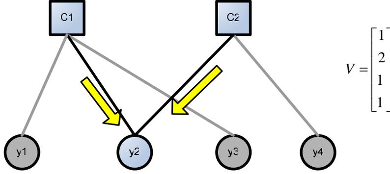
**Figure 4** Example of the averaging operation at each sensor node. The vector  $V$  represents the degree of each sensor node.
