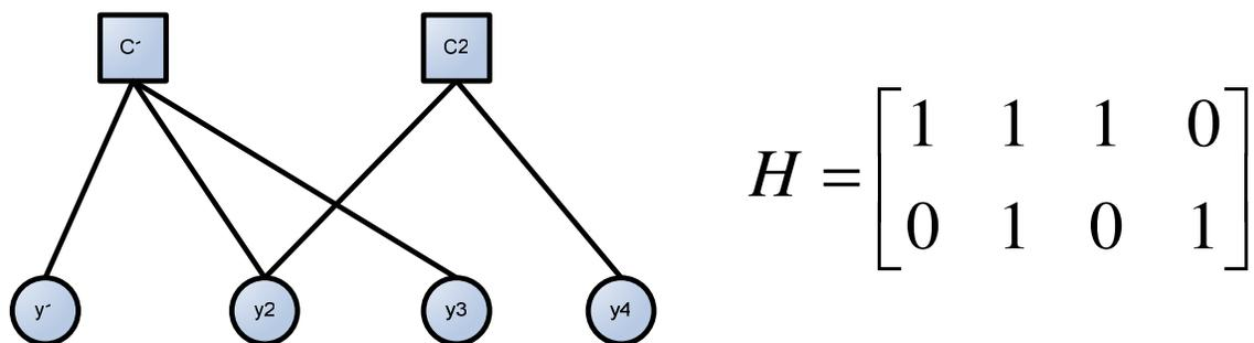
Figure 1 Representation of WSN using Tanner graph and parity check matrix.
