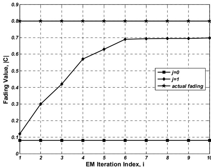
Figure 4. Change in estimated fade values versus actual fading value for the  $p^{\text{th}}$  subframe, where  $p = 48$  at  $E_b/N_0$  of zero dB (see the appendix for computer program number 1).
