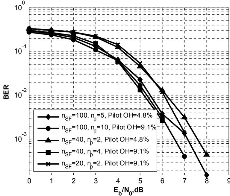
Figure 5. BER versus  $E_b/N_0$  for BPSK, for block length  $n = 2,000$  bits and receiver iterations  $j = 9$  with pilot overhead and number of code symbols as parameters for correlated Jakes fading with normalized fade rate of 0.005 (see the appendix for computer program number 1).
