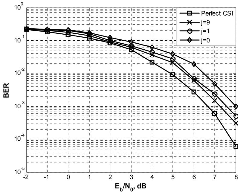
Figure 8. BER versus  $E_b/N_0$  for QPSK, for block length  $n = 2,000$  bits and receiver iterations  $j = 0, 1, 3$  and  $9$  with 9.1 percent pilot symbol overhead for correlated Jakes fading with normalized fade rate of 0.005 (see the appendix for computer program number 3).
