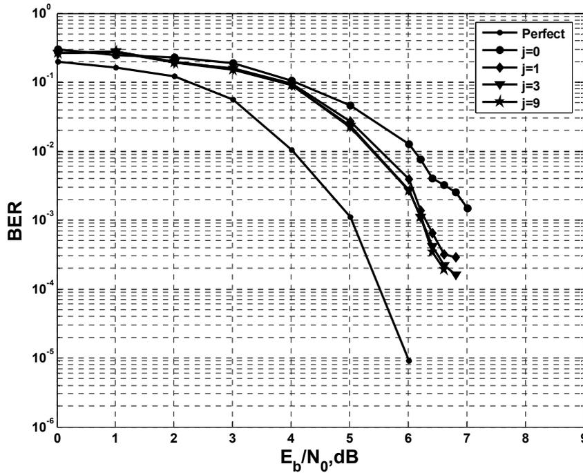
Figure 7. BER versus  $E_b/N_0$  for BPSK, for block length  $n = 2,000$  bits and receiver iterations  $j = 0, 1, 3,$  and  $9$  with 9.1 percent pilot symbol overhead for uncorrelated Rayleigh fading (see the appendix for computer program number 2) .
