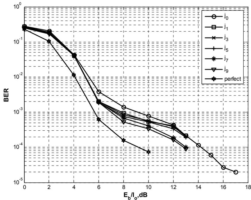
Figure 10. BER versus  $E_b/I_0$  for BPSK, for block length  $n = 2,000$  code bits and receiver iterations  $j = 0, 1, 3, 5, 7,$  and  $9$  with adaptive  $I_0$  and fading coefficient estimation for independent Rayleigh block fading (see the appendix for computer program number 4).
