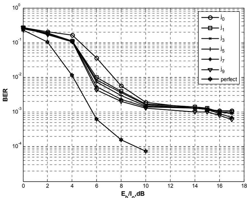
Figure 11. BER versus  $E_b/I_0$  for BPSK, for block length  $n = 2,000$  code bits and receiver iterations  $j = 0, 1, 3, 5, 7,$  and  $9$  with non-adaptive  $I_0$  and fading coefficient estimation for independent Rayleigh block fading (see the appendix for computer program number 5).
