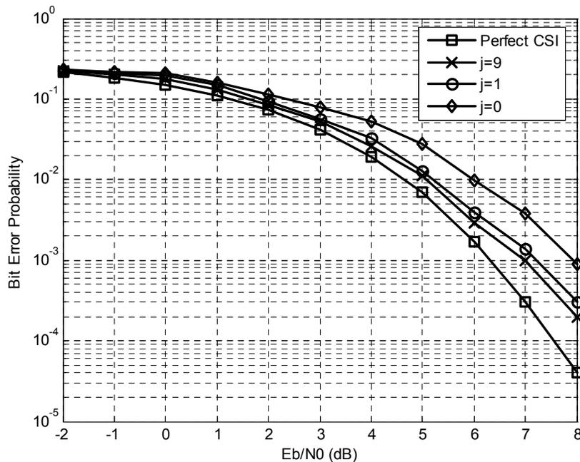
Figure 9. BER versus  $E_b/N_0$  for QPSK, for block length  $n = 2,000$  bits and receiver iterations  $j = 0, 1, 3$ , and  $9$  with 9.1 percent pilot symbol overhead for uncorrelated Rayleigh fading (see the appendix for computer program number 3).
