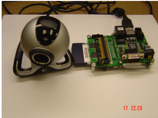
Figure 1.2: This figure shows the stargate sensor board connected to a web camera that together form an image sensor node.
