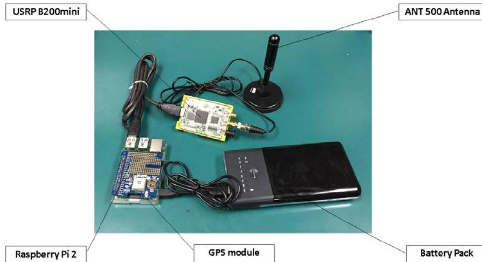
Figure 3.2: Spectrum sensing device prototype
