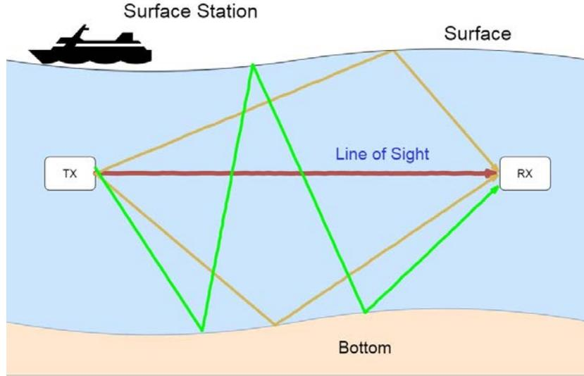
Figure 5.1: Underwater Acoustic Communication Channel under Multipath Effects
