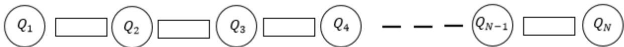
Figure 4.1. Linear nearest neighbor array comprising of N-qubits. Circles represent qubits and rectangles represent couplings between adjacent qubits. Each qubits can only interact with its nearest neighbors.
