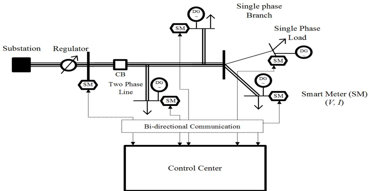
Figure 5 Distribution feeder with DG's, communication and control center [32].
