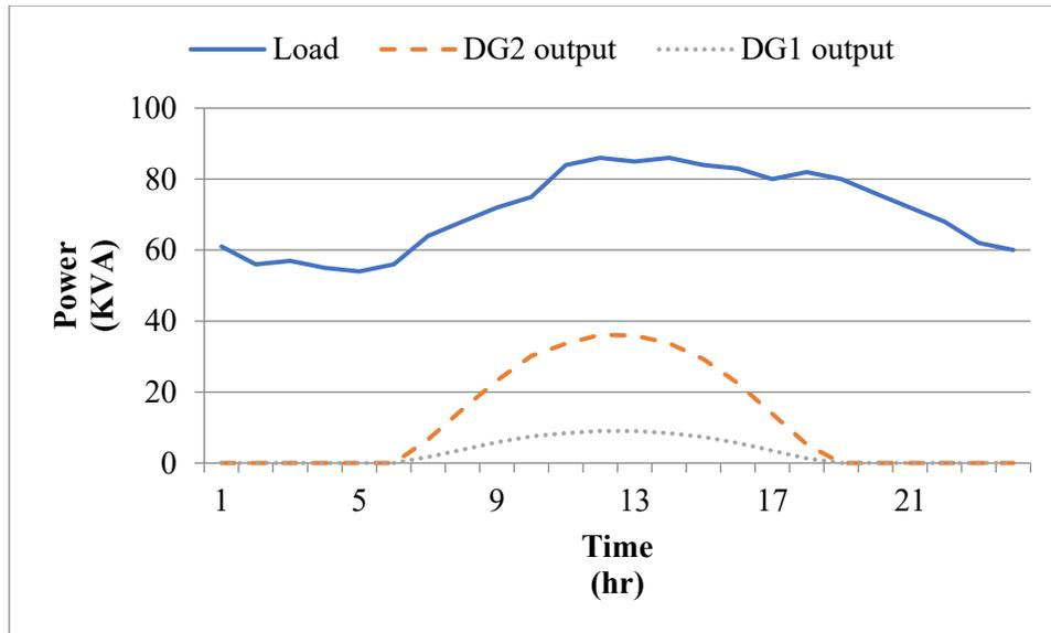
Figure 14 Load and PV generator profiles.
