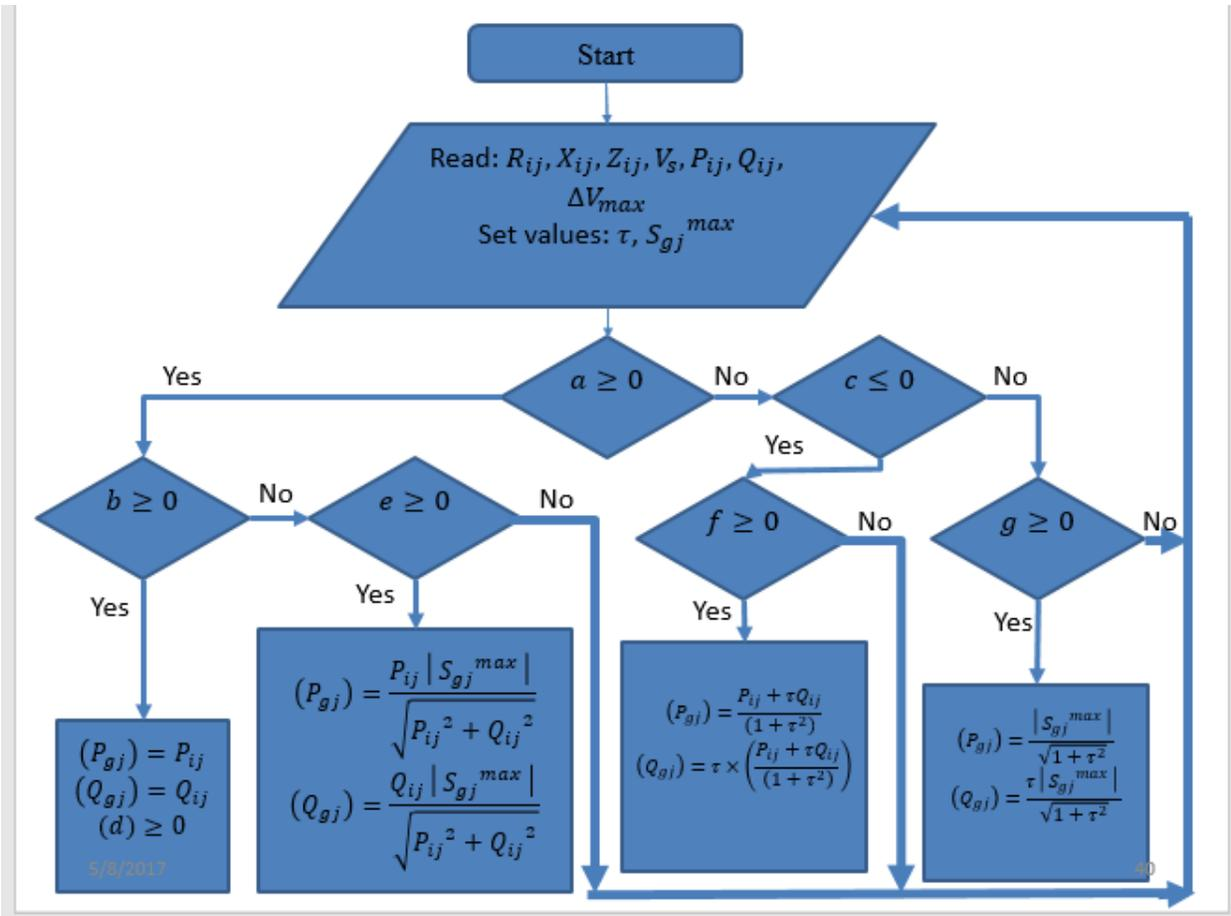
Figure 12 Flowchart algorithm for DG output.
