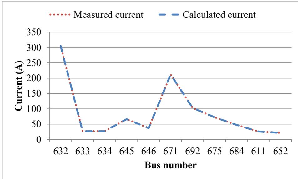
Figure 8 Line current analytical vs simulation.
