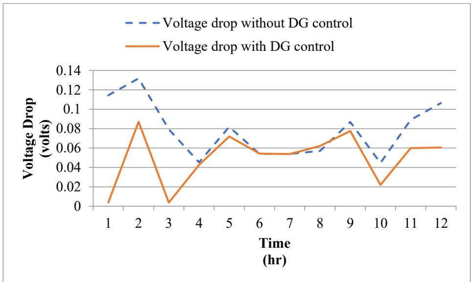
Figure 16 Voltage drop comparison for the line 692-675.
