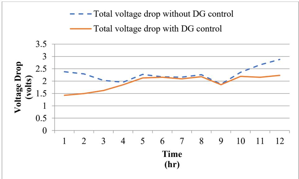
Figure 17 Total feeder voltage drop comparison.
