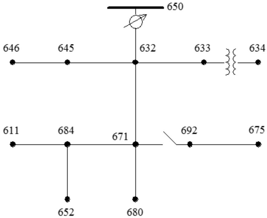
Figure 7 IEEE 13 node test feeder 1 [33].
