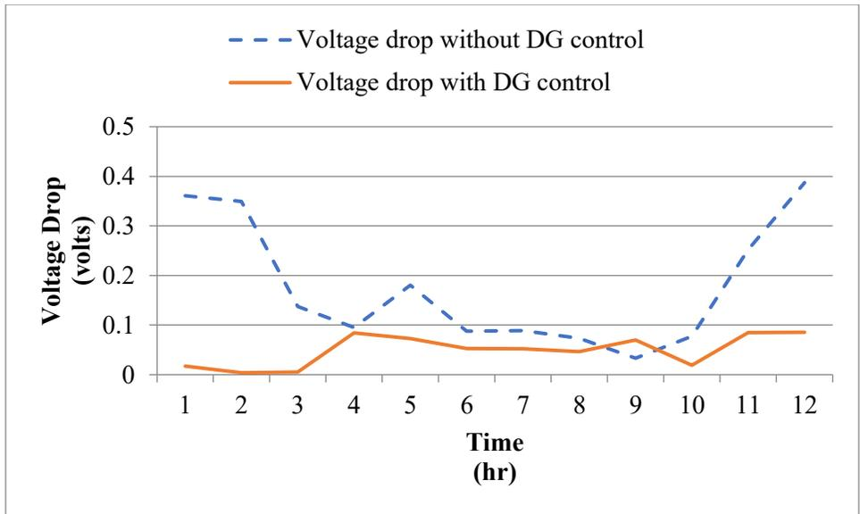
Figure 15 Voltage drop comparison for the line 632-671.
