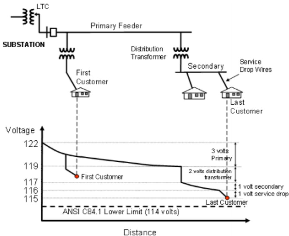
Figure 3 Distribution feeder first and last customer voltages [4].
