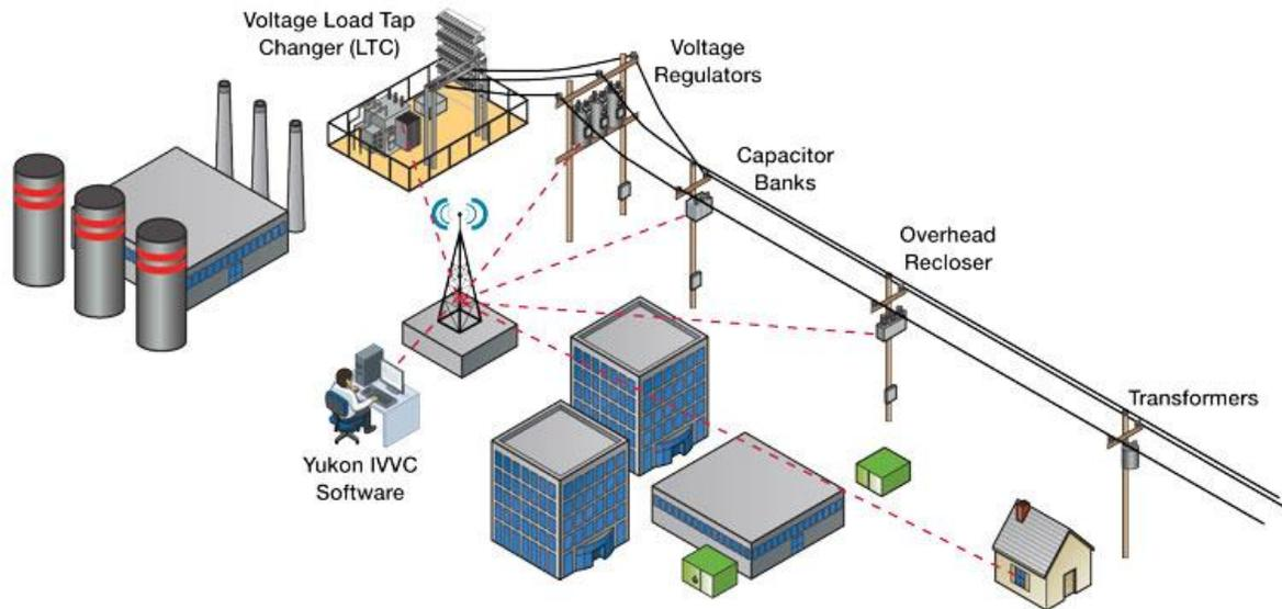
Figure 4 Distribution system voltage regulating devices [14].
