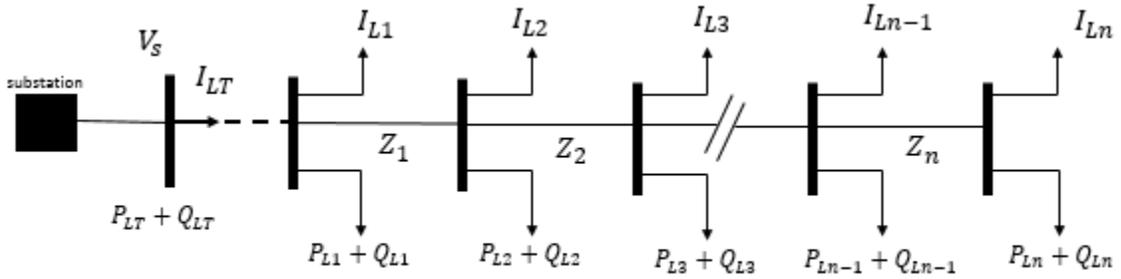
Figure 6 Radial distribution feeder 1.
