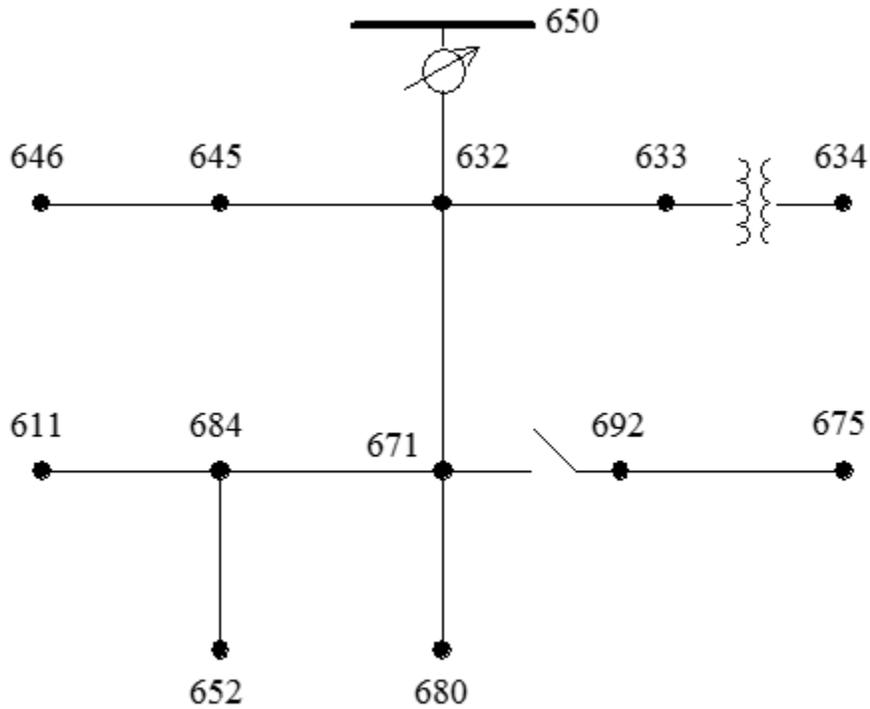
Figure 13 IEEE 13 node test feeder 2 [33].
