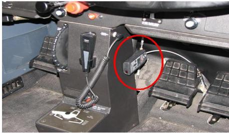
Fig.1. The location of instrument panel CO detector in GA cabin
