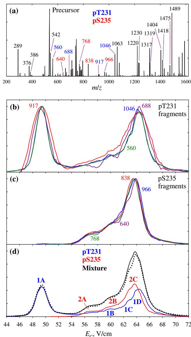
**Figure 1.** FAIMS/ETD data (with  $N_2$  buffer) for the  $pT^{231}/pS^{235}$  mixture: **(a)** total ETD spectrum with  $c/z$  fragments labeled (unique fragments color-coded); **(b), (c)** normalized spectra for all UF of  $pT^{231}$  and  $pS^{235}$  with the  $m/z$  values as marked; **(d)** measured trace (line) with the scaled spectra for both species produced by summing the spectra for all UF of each (above), and the mixture spectrum reconstructed by adding the two (dotted line)
