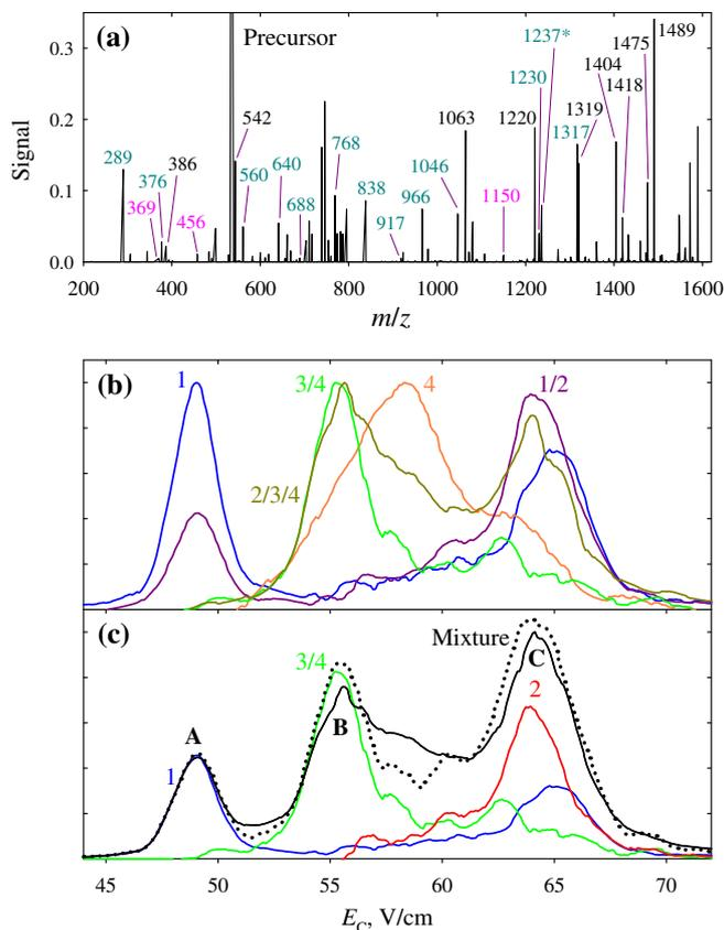
Figure 3. FAIMS/ETD data (with N<sub>2</sub> buffer) for the four-variant mixture: (a) total ETD spectrum with *c/z* fragments labeled; (b) normalized spectra for the precursors or their groups derived by summing the spectra for all distinguishing fragments; (c) measured trace (line) with the scaled spectra for individual species derived from above data, and the mixture spectrum obtained by adding them all (dotted line)
