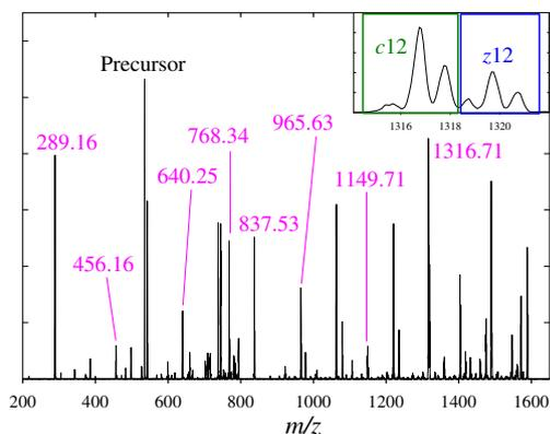
**Figure 5.** ETD spectrum measured at the peak B2 of Figure 4b in the normal mode
