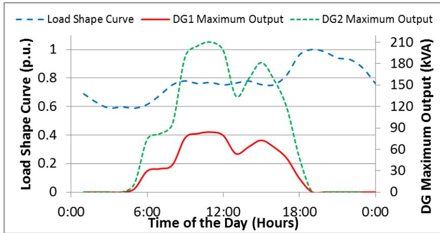
Figure 5.2: Load shape and DG output curves for 24 hours
