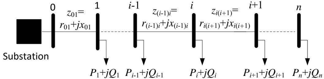
Figure 3.2: Radial Distribution System
