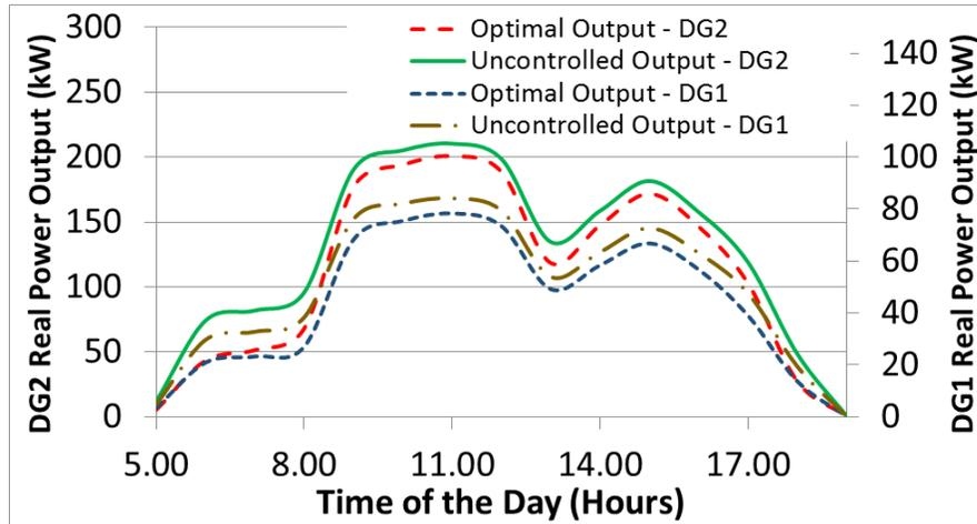
Figure 5.4: Real Power Outputs for node 1 and node 3
