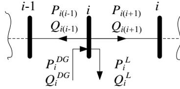
Figure 4.1: feeder sections connected to node i
