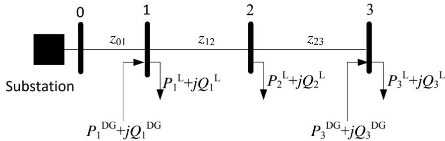
Figure 5.1: IEEE four node distribution test feeder
