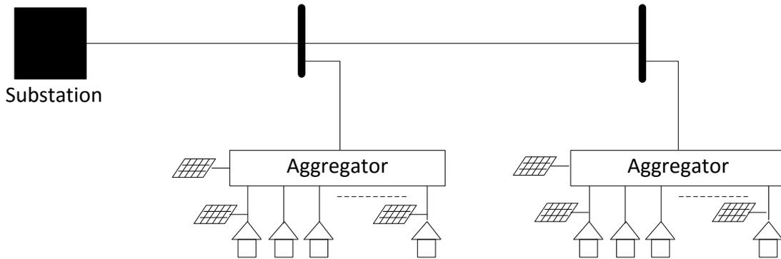
Figure 3.1: Aggregator Based Radial Distribution System with Co-Located PV
