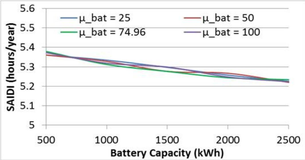
Figure.17: Effect of repair rate and battery capacity on SAIDI
