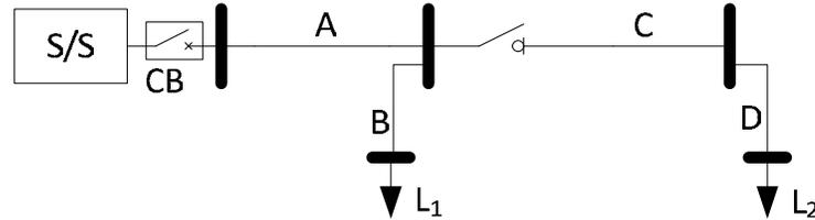
Figure.7:A simple two node feeder
