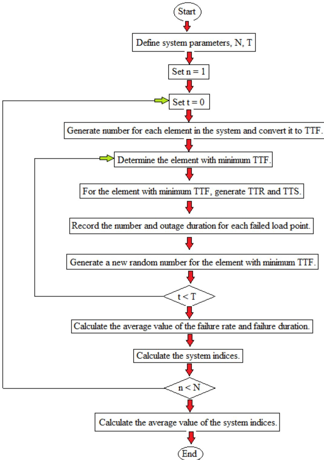
Figure.5: Flow chart of time Sequential Monte Carlo Simulation Technique
