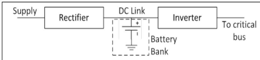
Figure.10: Non-redundant uninterruptible power supply.
