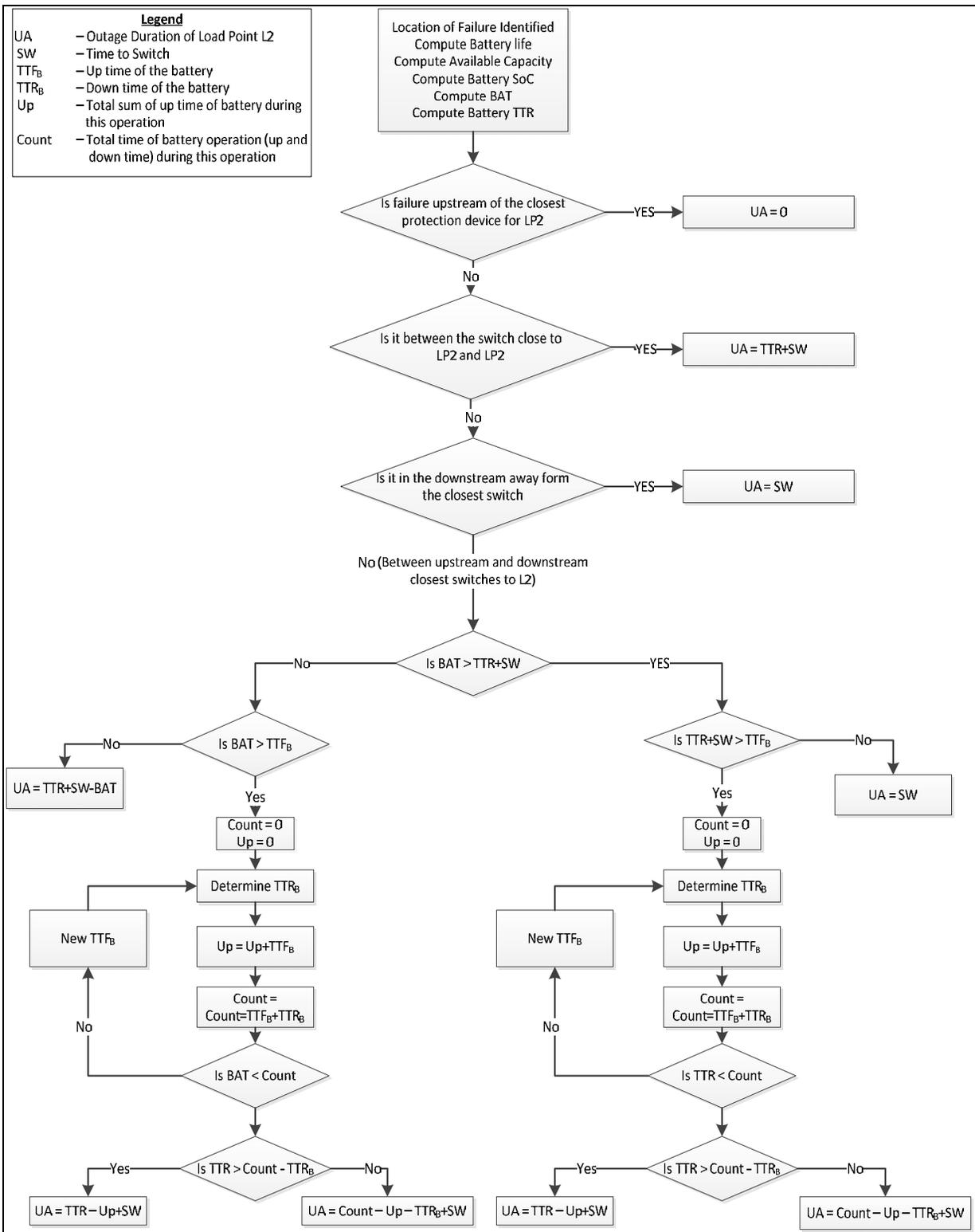
Figure.13: Flowchart of outage computation algorithm for the load point collocated with battery
