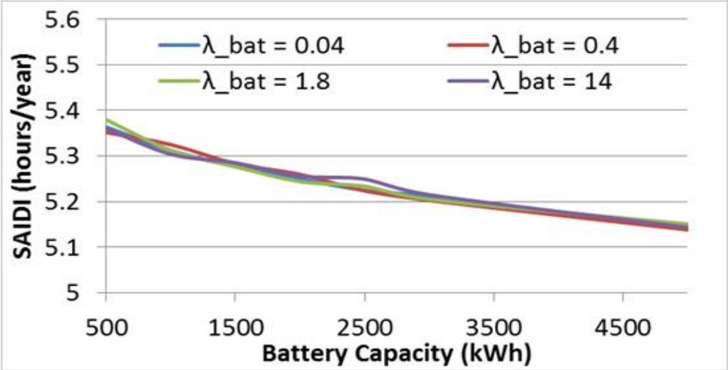
Figure.16: Effect of failure rate and battery capacity on SAIDI
