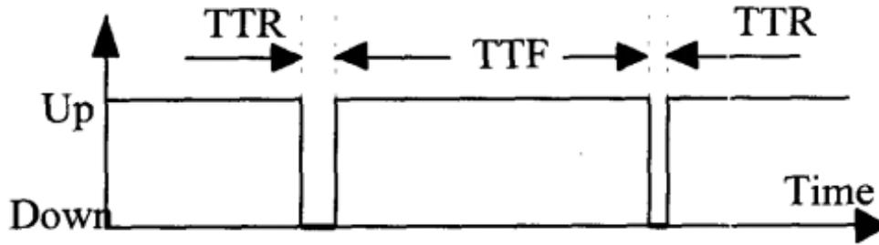
Figure.4: Component operating/repair cycles [19]
