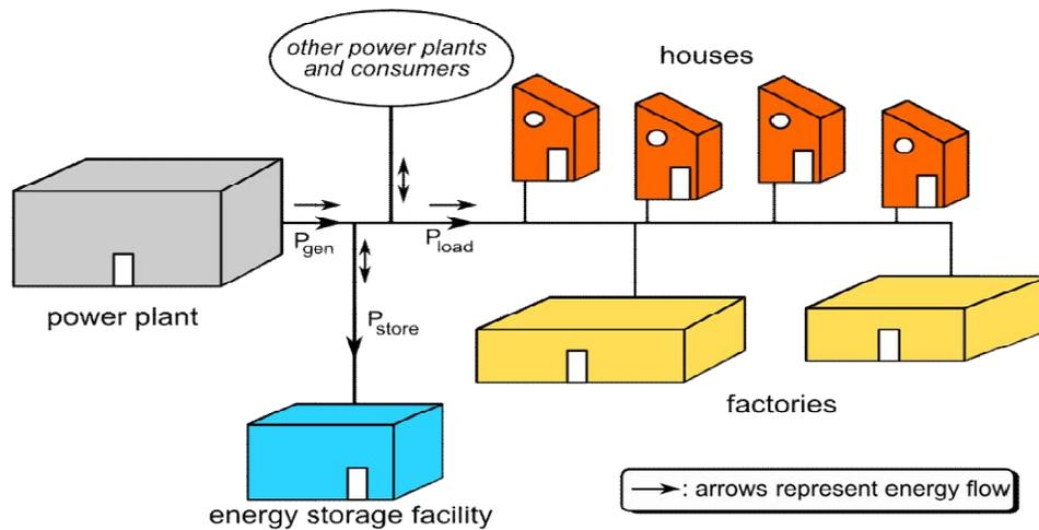
Figure.1: Energy Storage in a radial distribution network[7]
