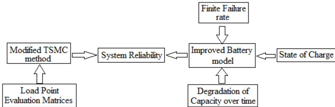
Figure 6: Flow chart of modeling methodology
