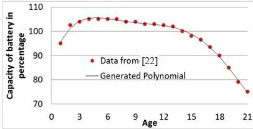
Figure.11: Battery Capacity vs. age
