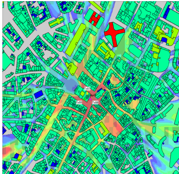
Figure 3.1: Urban micro-cell showing signal propagation and path loss in Karlsruhe, Germany. Strong signal areas are marked bright red, moderate signal strength is indicated by green, and no-signal areas are blue.
