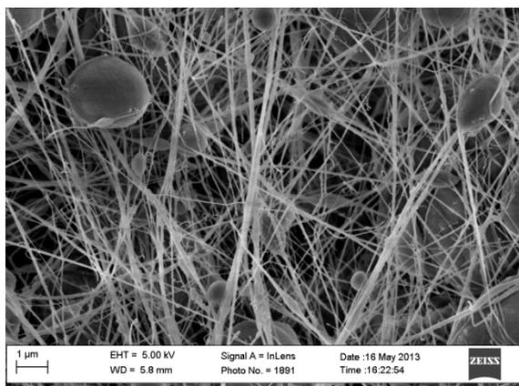
Fig. 1. The SEM image of PVdF/PVP with 4 wt% carbon black
