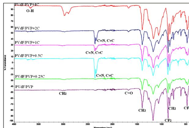
Fig. 3. The FTIR spectrum of PVdF/PVP with different percentage of carbon black
