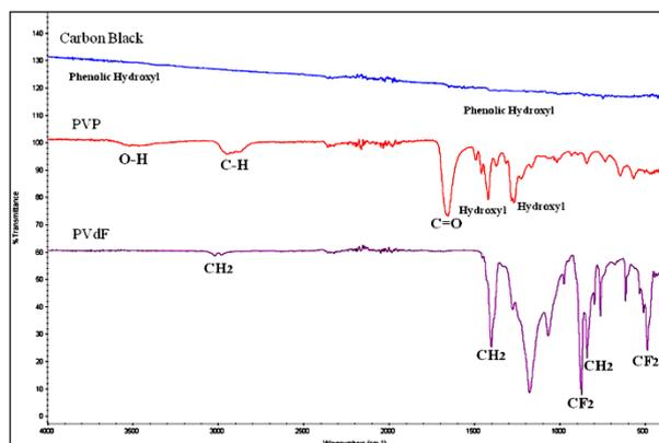
Fig. 2. The FTIR spectrum of pure PVdF, PVP and carbon black
