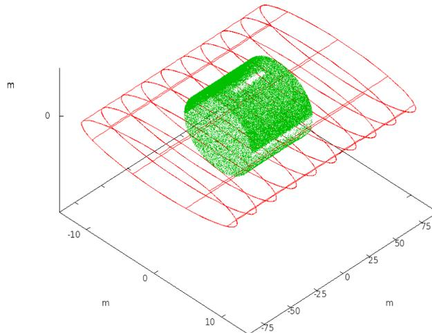
Figure 19: Elliptical Cylinder Volume Inside Submarine
