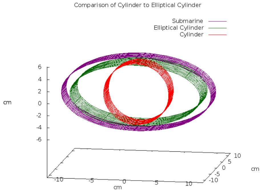
Figure 17: Side by Side Comparison of Cylindrical and Elliptical Volume vs Submarine Outline
