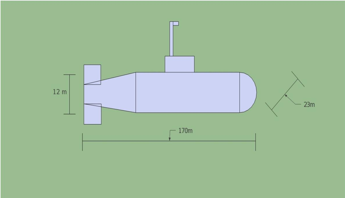
Figure 1: Dimensions of a Typhoon Class Submarine
