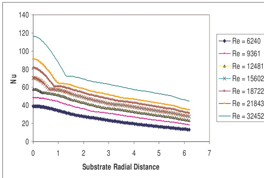
Figure14. Nusselt number along the substrate (with radiation).
