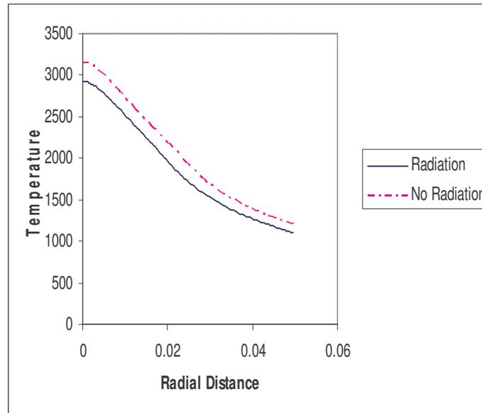
Figure 6. Temperature distribution along substrate radial direction.
