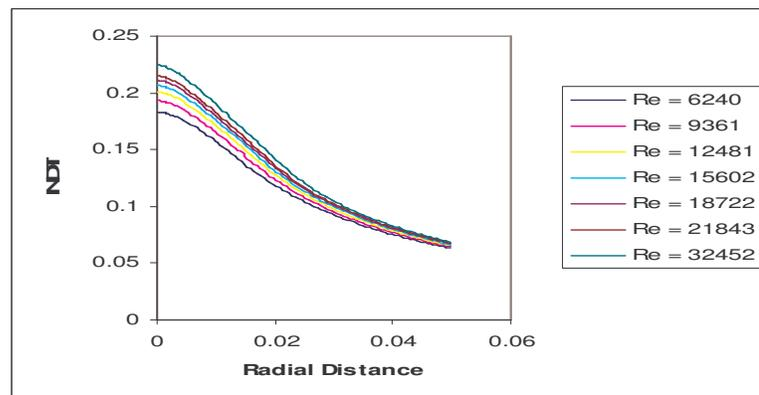
Figure 11. Distribution of non-dimensional temperature on the substrate (with radiation).
