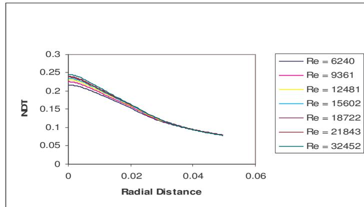
Figure 10. Distribution of non-dimensional temperature on the substrate (without radiation).
