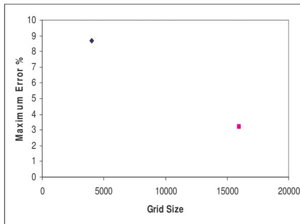
Figure 3. Error calculation for different grid sizes.
