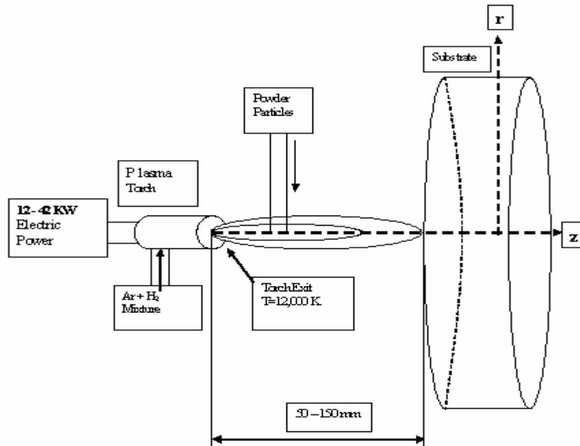
Figure 1. Schematic representation of typical plasma spray coating deposition system
