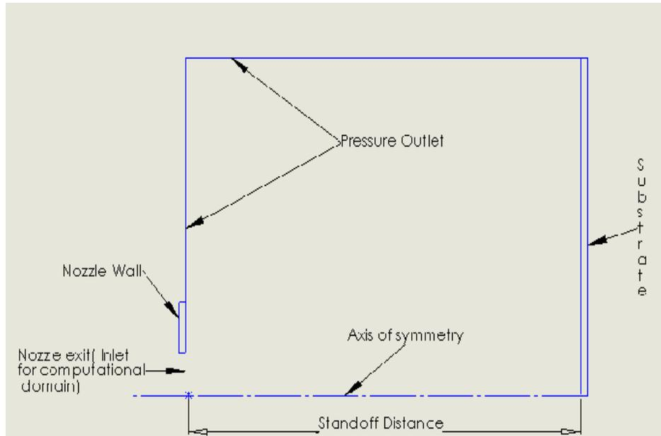
Figure 2. Computational domain for modeling plasma issuing into ambient air (nozzle exit radius 4 mm, nozzle wall thickness 8 mm, substrate radius 50 mm, stand-off distance 50 mm).
