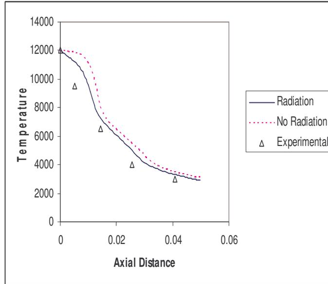
Figure 5. Temperature distribution along the jet axis.
