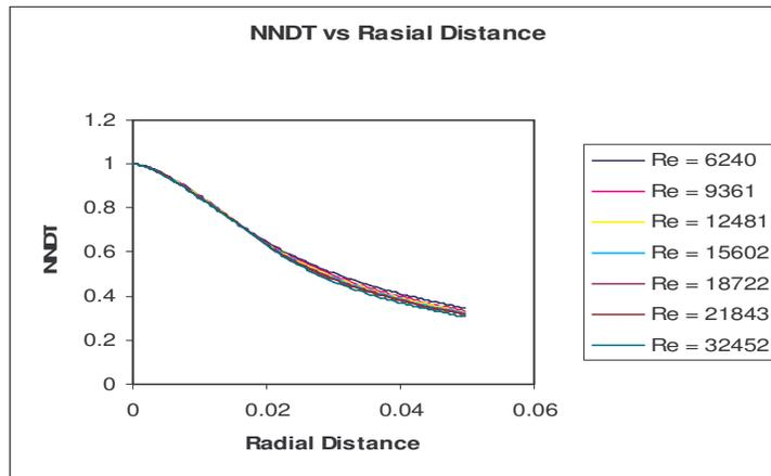
Figure 13. NNDT along the radial distance at substrate (with radiation).
