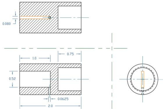
Figure (2): Test gripping mechanism.
