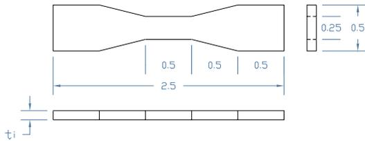
Figure (1): Test specimen geometry.
