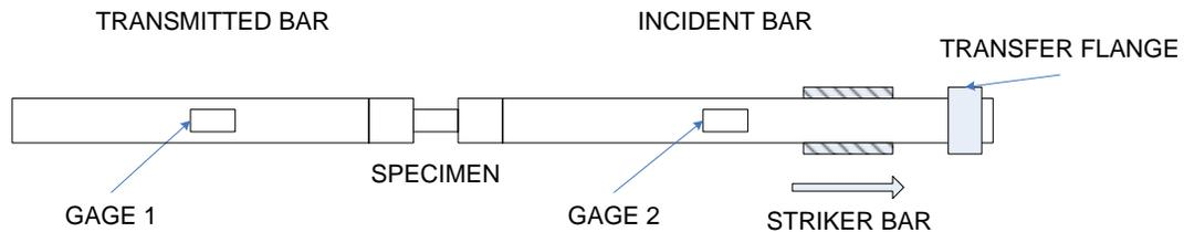
Figure (4): Tension Split Hopkinson Pressure Bar Apparatus.
