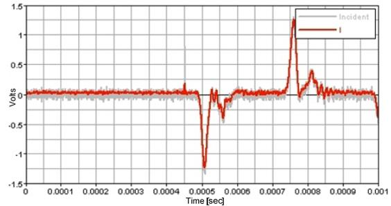
Figure (5): Incident pulse before and after dispersion correction.
