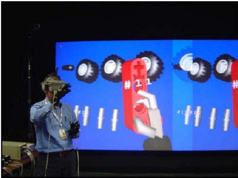
**Figure 2. A participant in the HMD Environment manipulates a virtual part. The participant's view of the environment can be seen on the screen in the background.**
