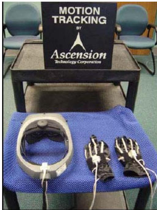
**Figure 1. HMD and pinch gloves with motion tracking sensor attached.**
