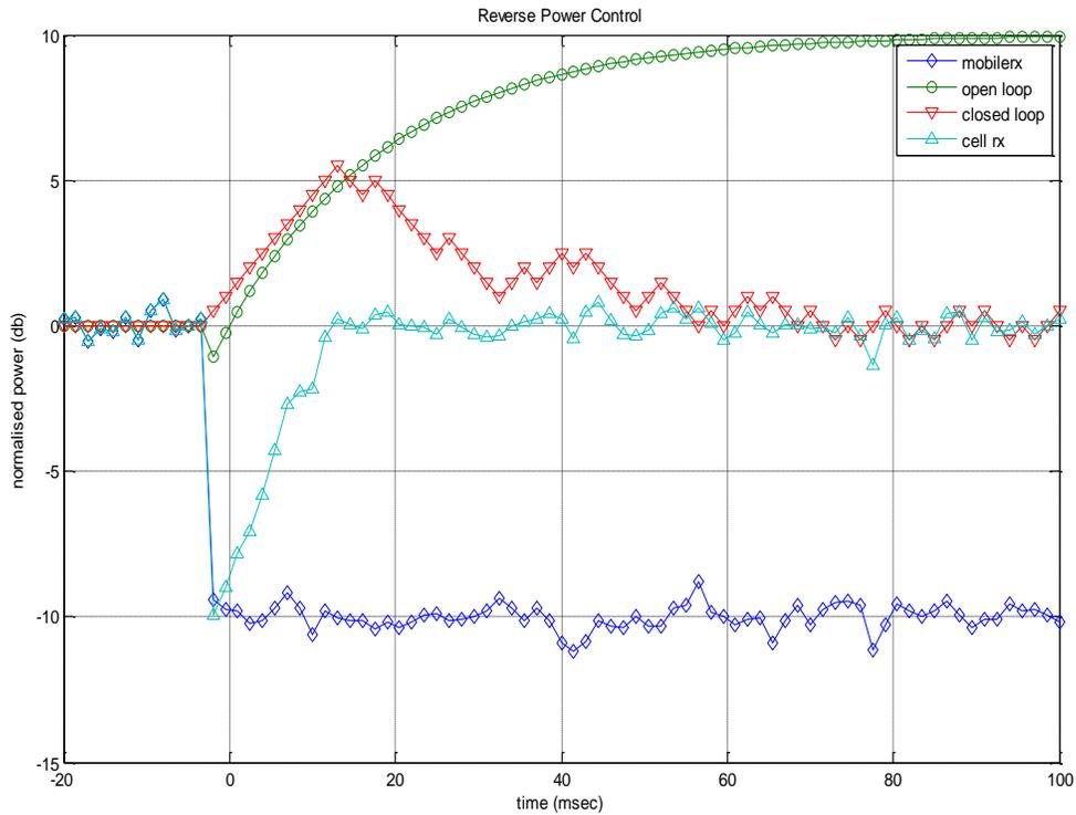
Figure 5. Reverse Power Control for Regular CDMA System.
