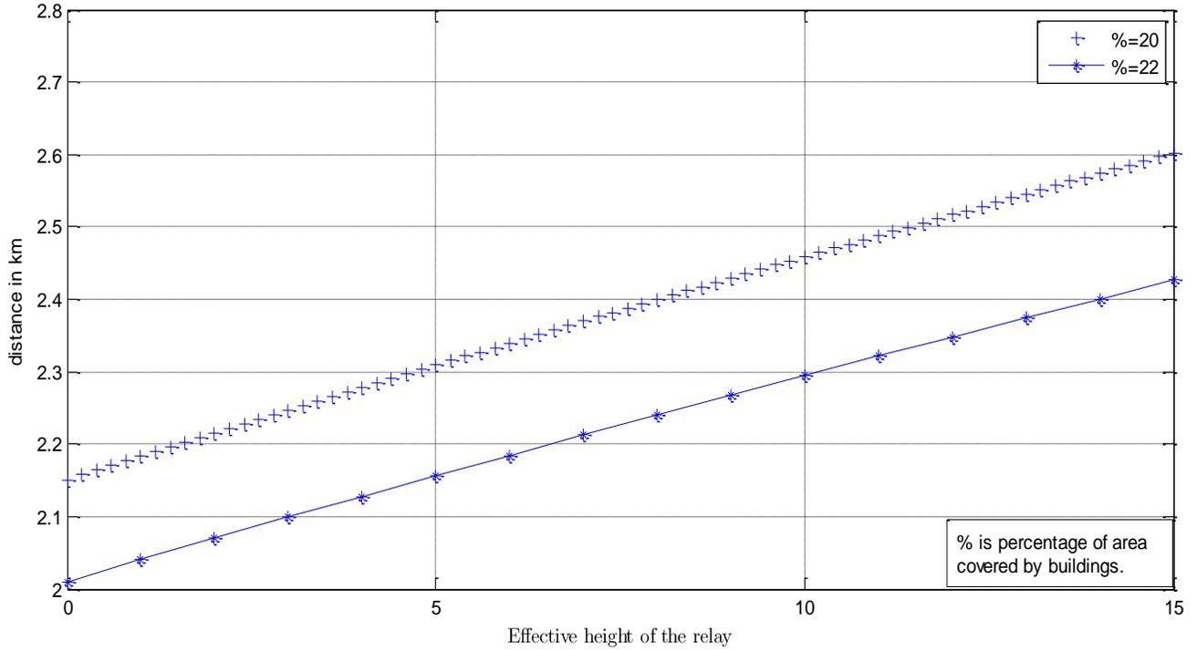
Figure 8. Distance in Kilometers Given Effective Height of Relay.
