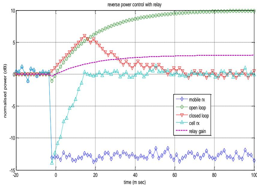
Figure 6. Reverse Power Control for Relay-Based CDMA System.
