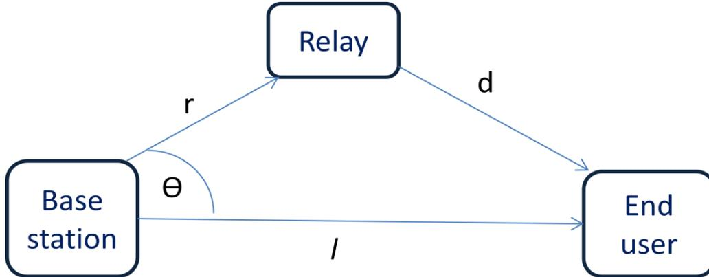
Figure 2. Simple Relay Network.
