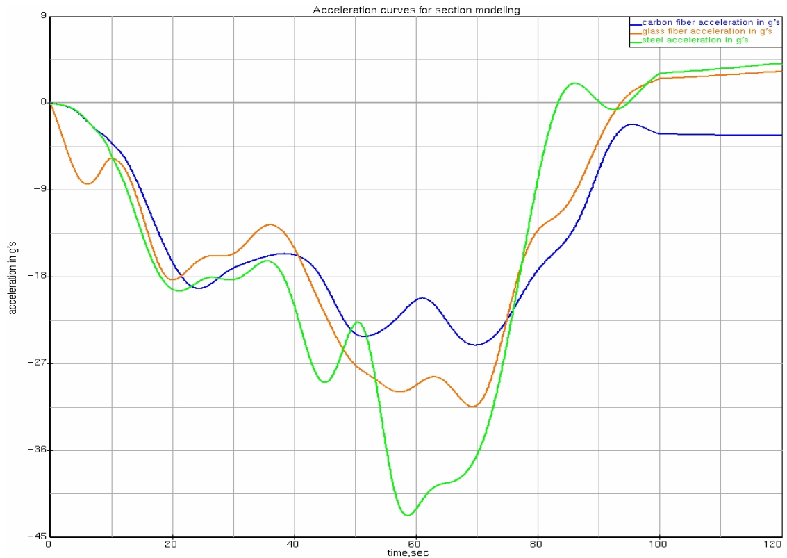
Figure 51. Comparison of acceleration curves of Centre of gravity for carbon fiber, glass fiber and steel.
