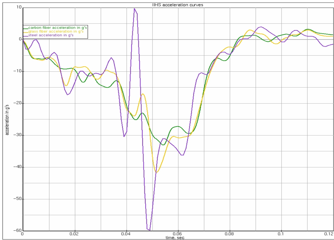
Figure 62. Comparison of acceleration curves of Centre of gravity for carbon fiber, glass fiber and steel.
