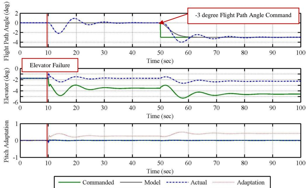
Fig. 1. Flight path angle and pitch neural network response to simulated 50% reduction in elevator effectiveness (10s), negative 3 degree flight path angle command (20 s), 50% reduction in thrust (90s) and 10 ft/sec increase in airspeed (100s)
