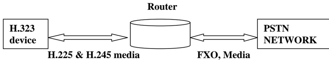
**Figure 2 - Protocols used by the gateway**
