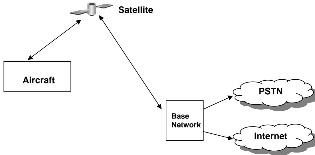
**Figure 4 Basic aircraft data network**
