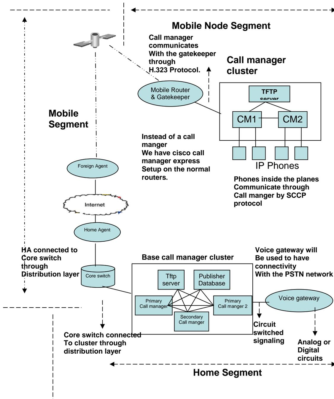
**Figure 10 Proposed model for voice communication on the aircraft**
